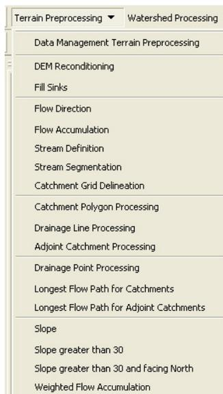
Figure 1. ArcHydro Terrain Preprocessing Menu
