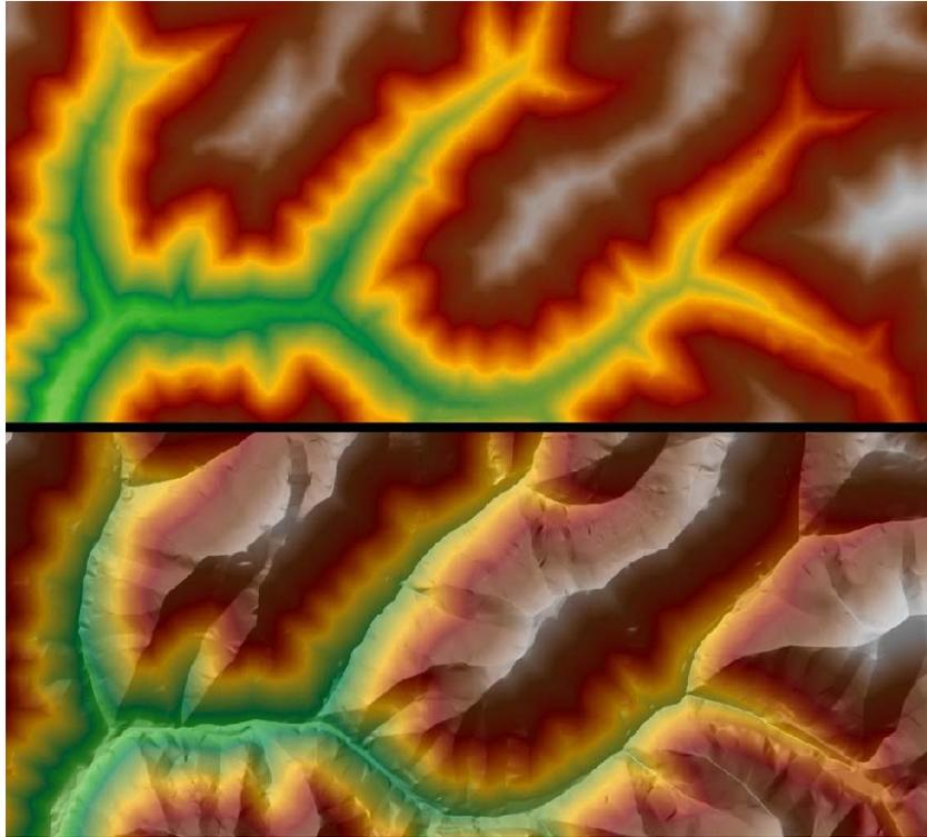
Figure 6. Hillshaded DTM to no hillshade comparison
