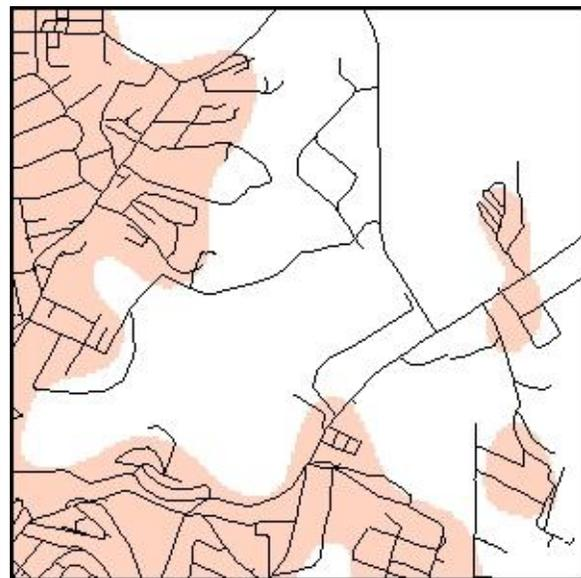
Figure 9 - Focal Raster, Annulus Neighborhood Shape, 2 cell Inner radius, 15 cell Outer radius
