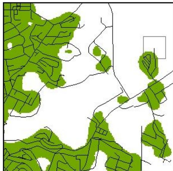
Figure 11 - Focal Raster, Annulus Neighborhood Shape, 2 cell Inner radius, 15 cell Outer radius
