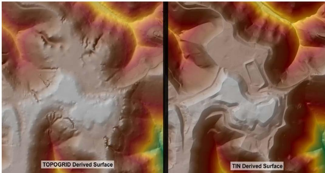
Figure 2. Comparison between TOPOGRID and TIN derived surfaces.
